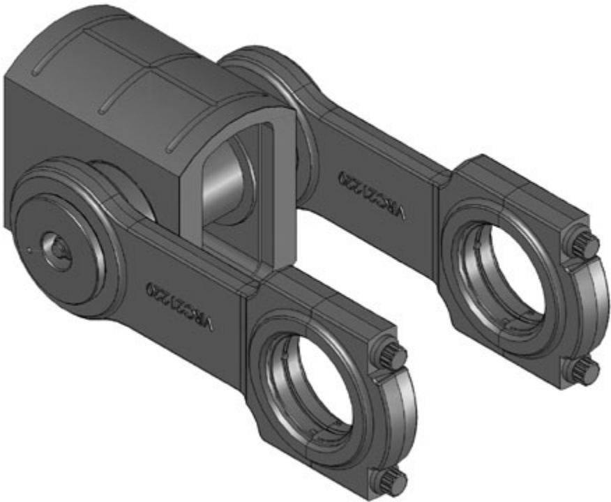
Figure 4.4- Crosshead and Double Light Connecting Rod Assembly
