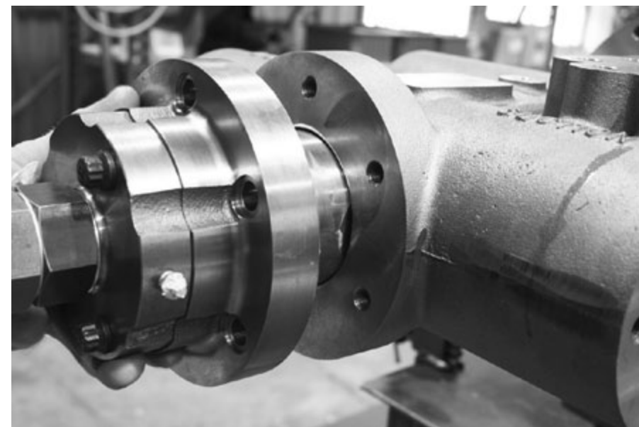
3. Push the VVCP into the cylinder.
