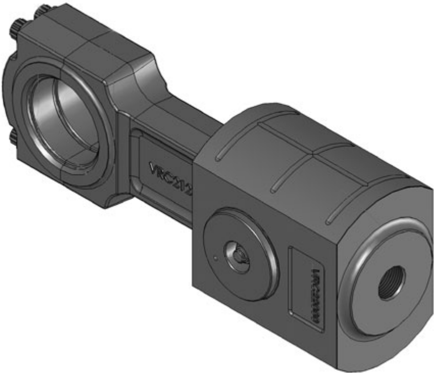
Figure 4.3- Crosshead and Single Heavy Connecting Rod Assembly
