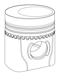
Place expander spacer in the oil ring groove with the ends of the spacer above the solid portion of the groove bottom.
