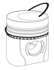
Install the other rail below the spacer, starting the rail 2" to the right of the spacer ends. Make sure the ends of the spacer are not overlapped. Do Not cut off the ends of the spacer.
