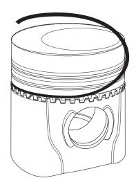
Holding the ends of the spacer butted together, install a steel rail on top of the spacer. Start the rail 2" to the left of the spacer ends and coil across the spacer ends and into the groove.
