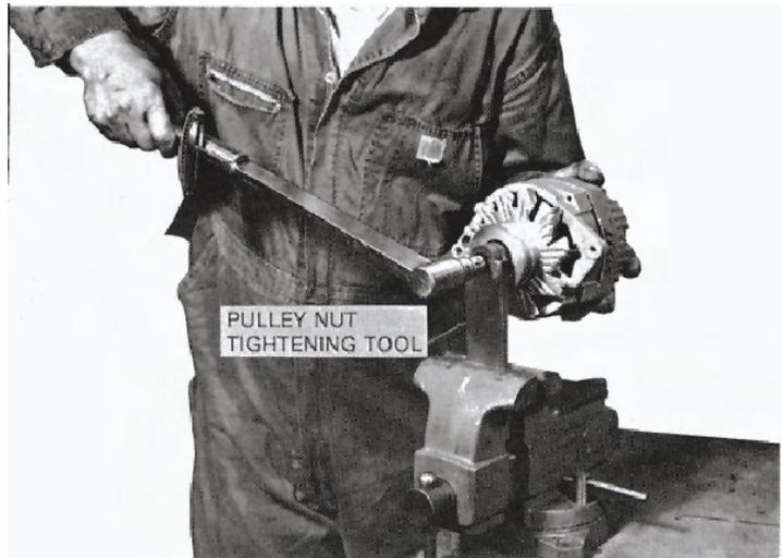
REMOVING THE ALTERNATOR PULLEY
