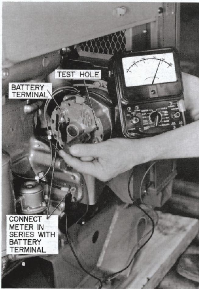
TESTING ALTERNATOR OUTPUT
