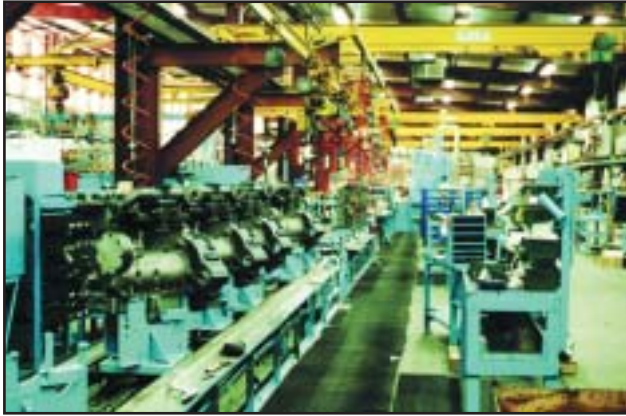
■ Arrow VR series engines are assembled on this conveyor line, which contains a block washer, rolover fixtures and other special tooling that can efficiently accommodate production runs of 10 or more engines at a time. Many of the engines are built as "long blocks" ready for short lead time completion with various customer preferred options.
