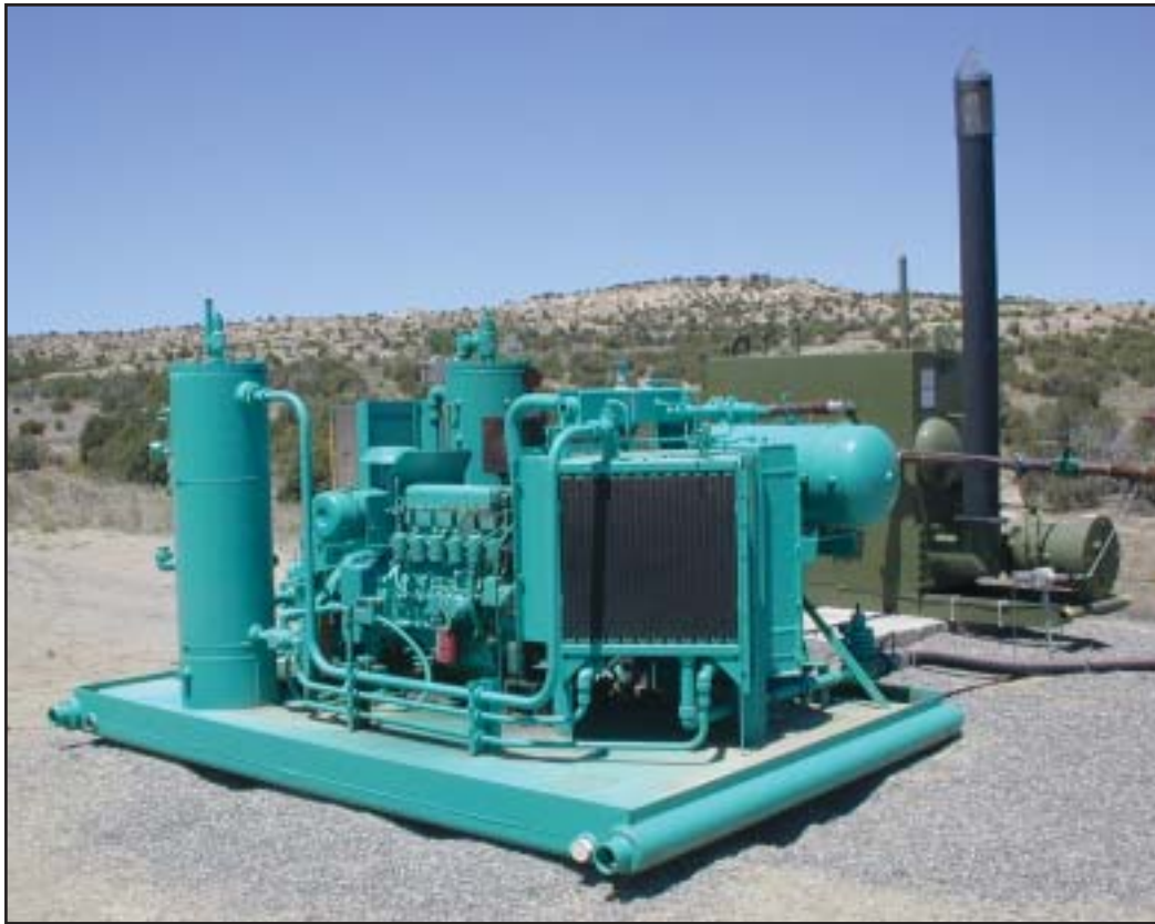
■ Arrow natural gas engines such as this VRG330 are popular in small horsepower gas compression applications in New Mexico and other gas patch areas.
