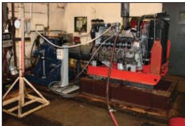
■ Each Arrow engine is factory tested on a dynamometer after assembly and before painting.
