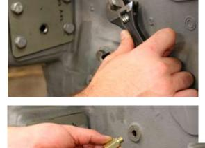
6. Remove plug from pressurized port located on left side of engine block. Replace plug with M10x1-to-1/8"NPT adapter. Attach 90° brass elbow with 1/8"NPT-to-5/16" tube fitting to adapter.
