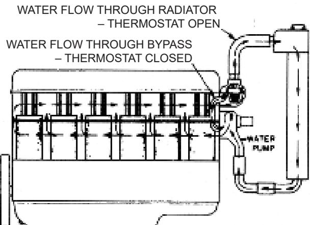
The thermostat regulates the engine temperature by automatically controlling the amount of coolant passing through the cooler or radiator core. Back pressure at the water outlet must not exceed 5 PSI (.35 kg/cm<sup>2</sup>).
