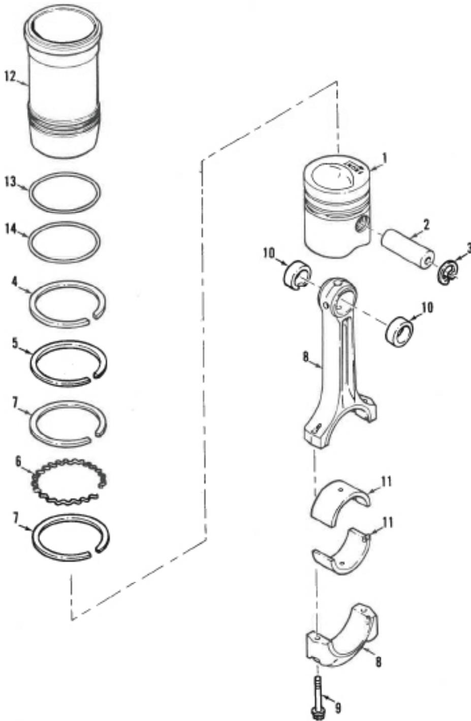
**PISTONS, CONNECTING RODS, CYLINDER SLEEVES**
