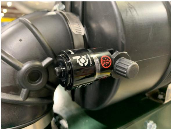
As dirt trapped by the air cleaner gradually restricts the flow of air, the condition indicator signal, which is preset for a maximum restriction, rises within the gauge. When the maximum restriction is reached, the signal locks into full view indicating the need for servicing the air cleaner element.
