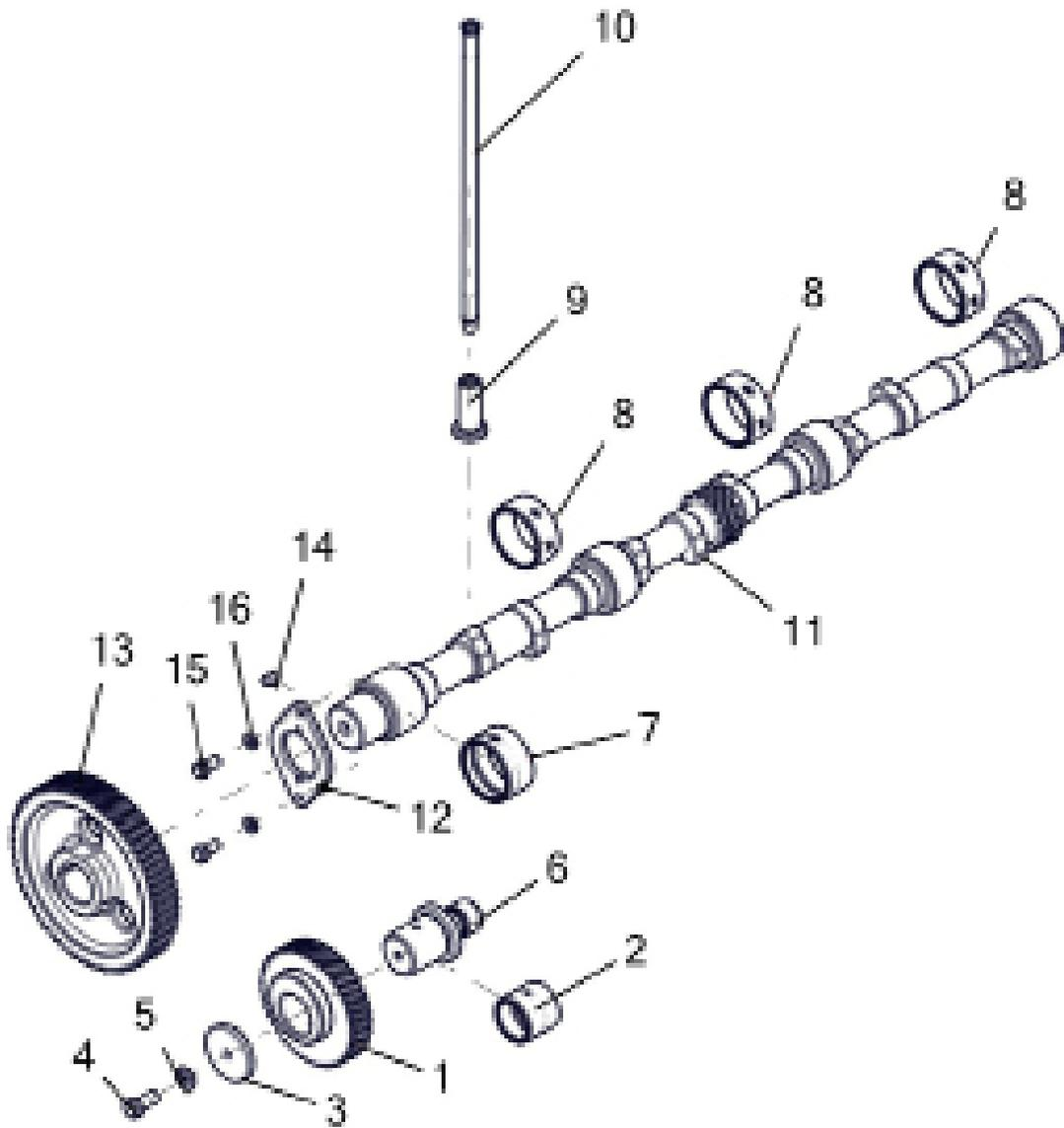
**CAMSHAFT, VALVE LIFTER, PUSH ROD, IDLER GEAR**
