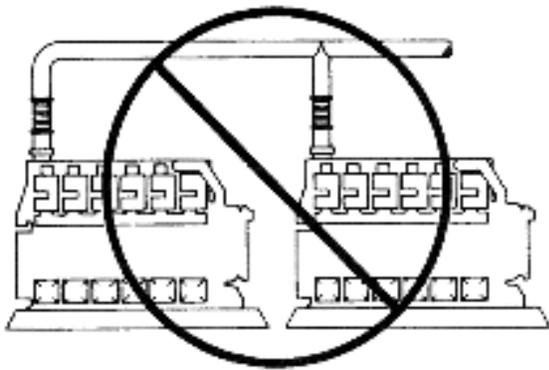
It is advantageous in every installation to locate the silencer as close to the engine as possible.
