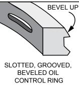
Oil compression rings are grooved, slotted, and beveled. The side with the **BEVEL** should be facing **UP**.
