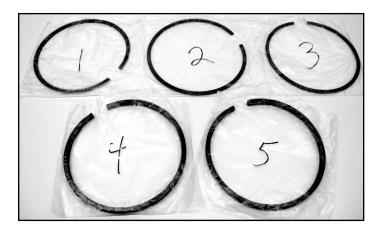
Rings cannot be interchanged. They are labeled in the package in the order they should be installed. New cylinder bores must be conditioned properly using bore deglaze. The glazed cylinder wall causes rings to "skate" on the highly polished finish and discourages the minute amount of wear which is necessary to mate piston rings with the bore.
