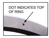
These compression rings are directional, meaning they have a top and bottom. The side with the **DOT** should be facing **UP**.
